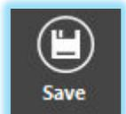
If you are editing the depths of a photo record, the Save button is required to be pressed to commit the changes and rename the photo. When not editing the depths, pressing the Save button will result in a new row with the same depths, but an incremented photo\_name being added to the DRILL\_HOLE\_CORE\_PHOTOS table.
